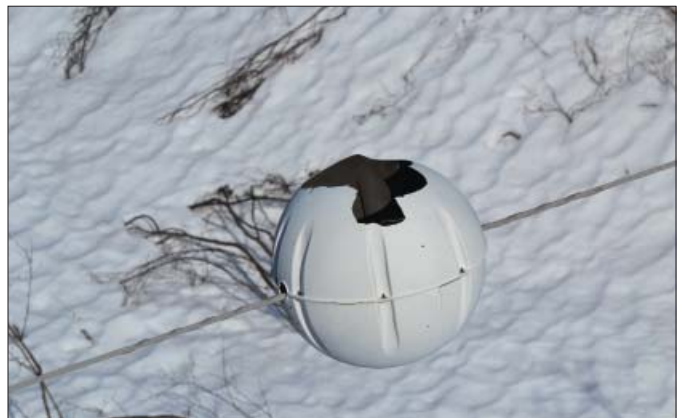
Top left, marker ball with bullet holes and frayed wire from being hit by bullets Top right, a brightly colored marker ball stands out against the surrounding terrain to demonstrate the location of the line Middle, marker balls crossing a span of line over a gorge between structures Bottom, a damaged marker ball
