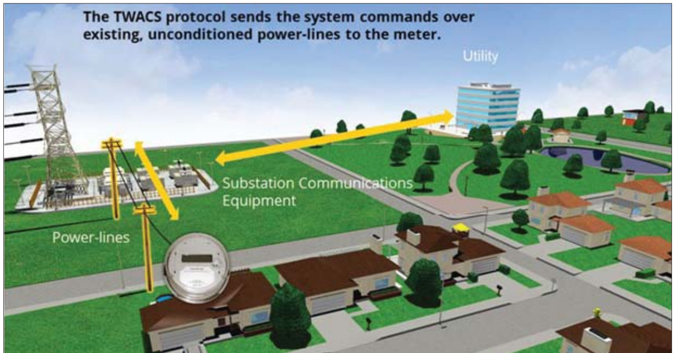
Above, the photo above depicts the flow of information using automated meters. Opposite, a picture of an automated meter, similar to what will be installed on the CVEA system
