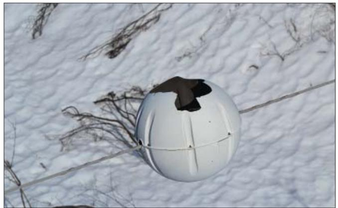
**Top left, marker ball with bullet holes and frayed wire from being hit by bullets
