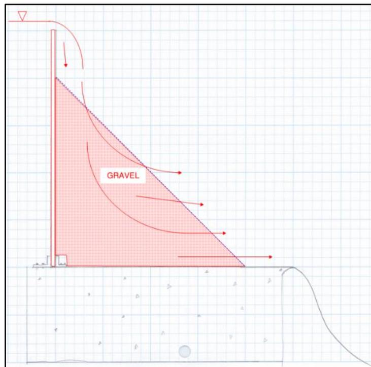
**Figure 4-4. Gravel ballast fuse gate**
