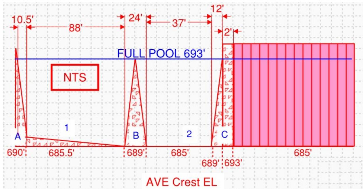
**Figure C-1. Section view of compound spillway**
