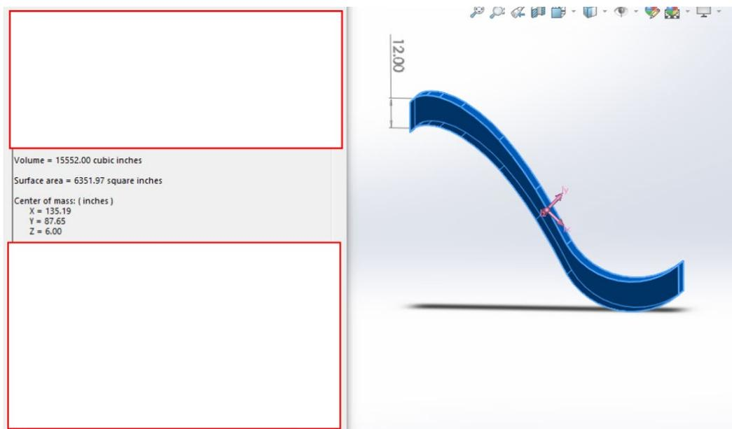
**Figure A-1. Properties of new concrete for a 1-foot raise over 1 foot of span**
