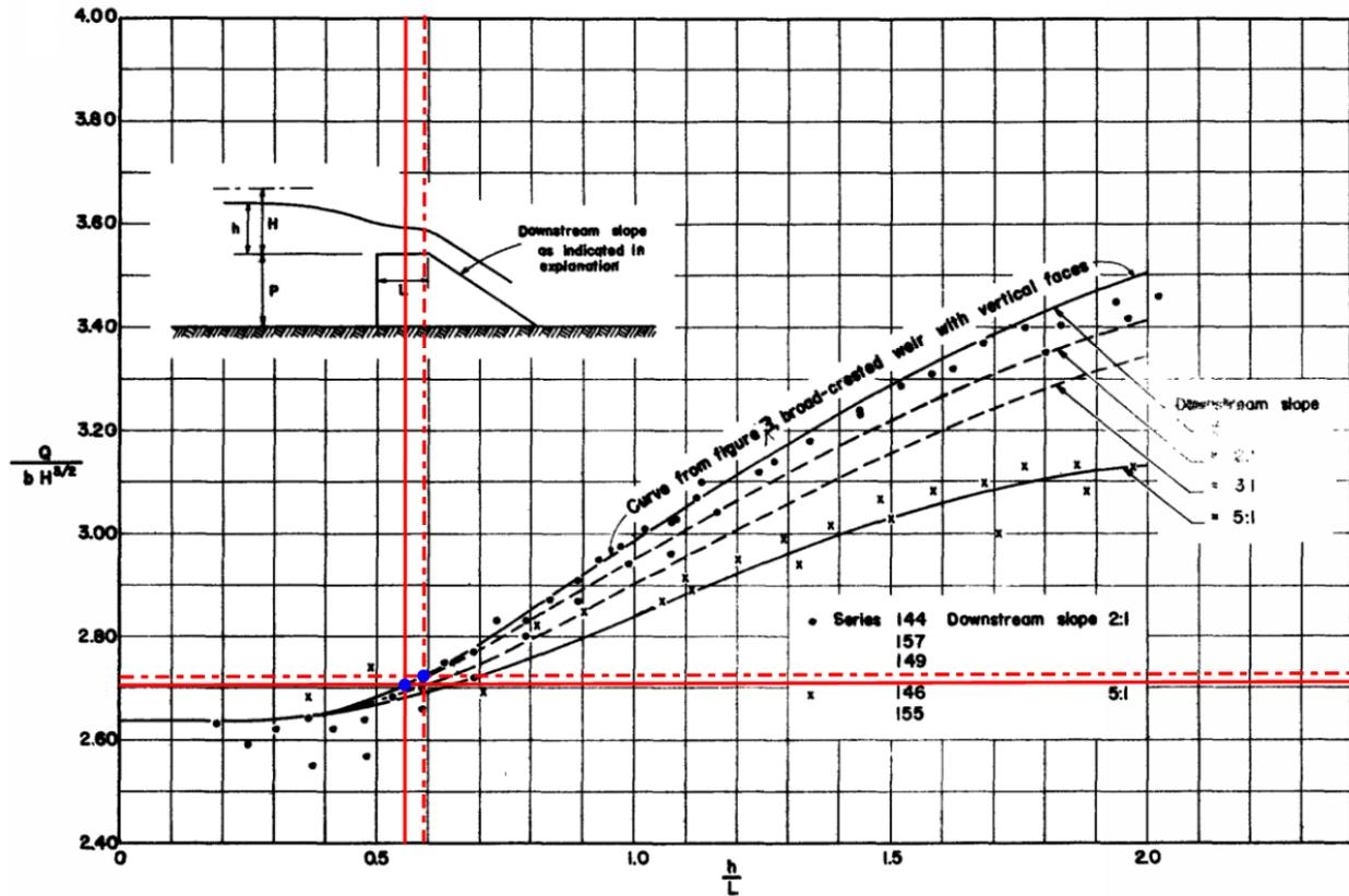
**Figure B-2. Determination of discharge coefficients for rubber dam sections during PMF**
