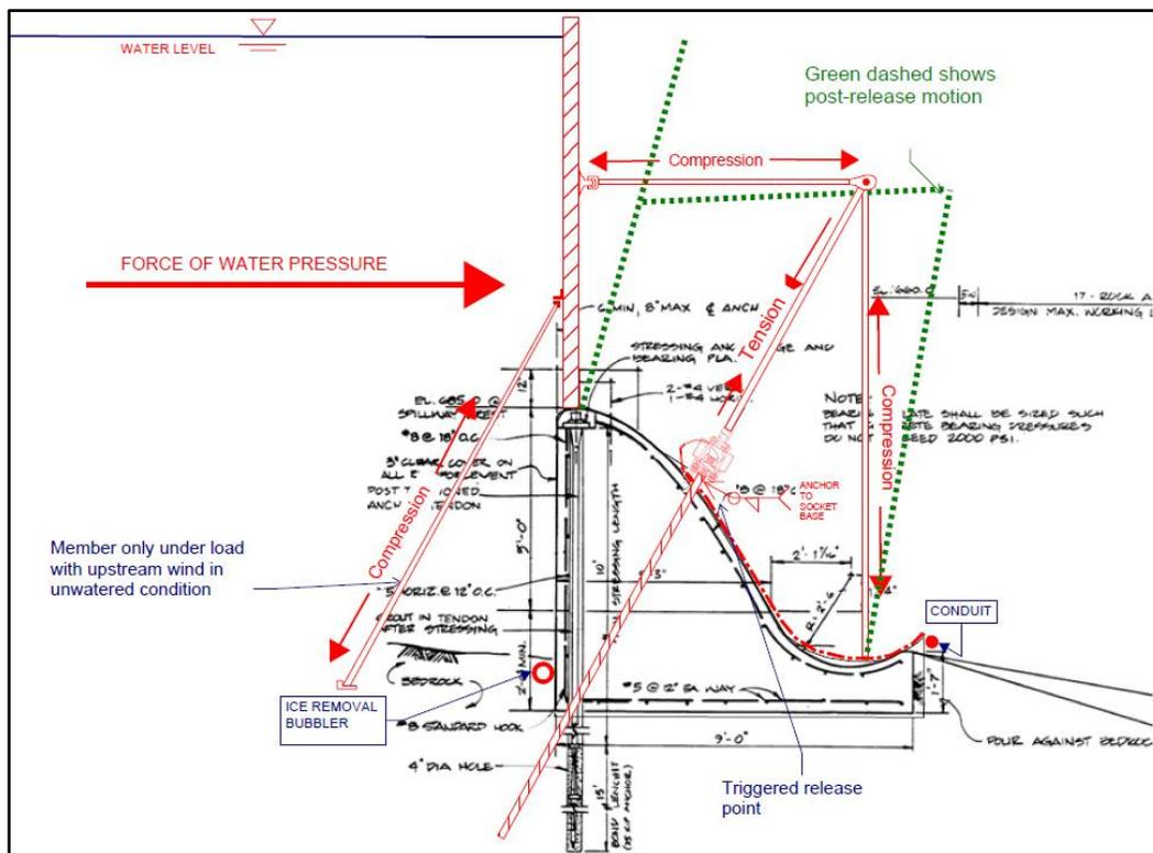
**Figure 4-7. Flashboards with frangible nut release on tension member**
