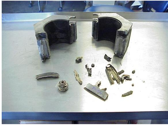
**Shuttle Frangible Nut Post-Function Test**
