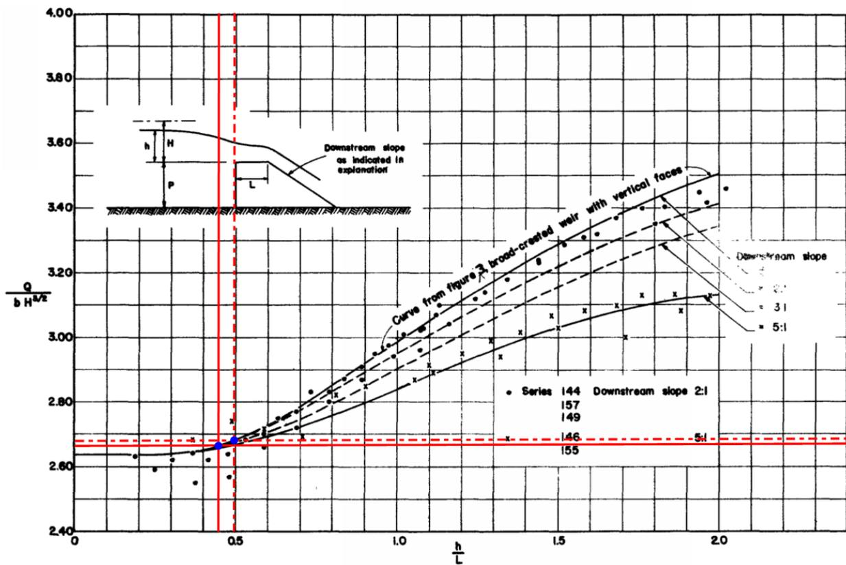
**Figure C-2. Determination of discharge coefficients for rubber dam sections at full pool water level**
