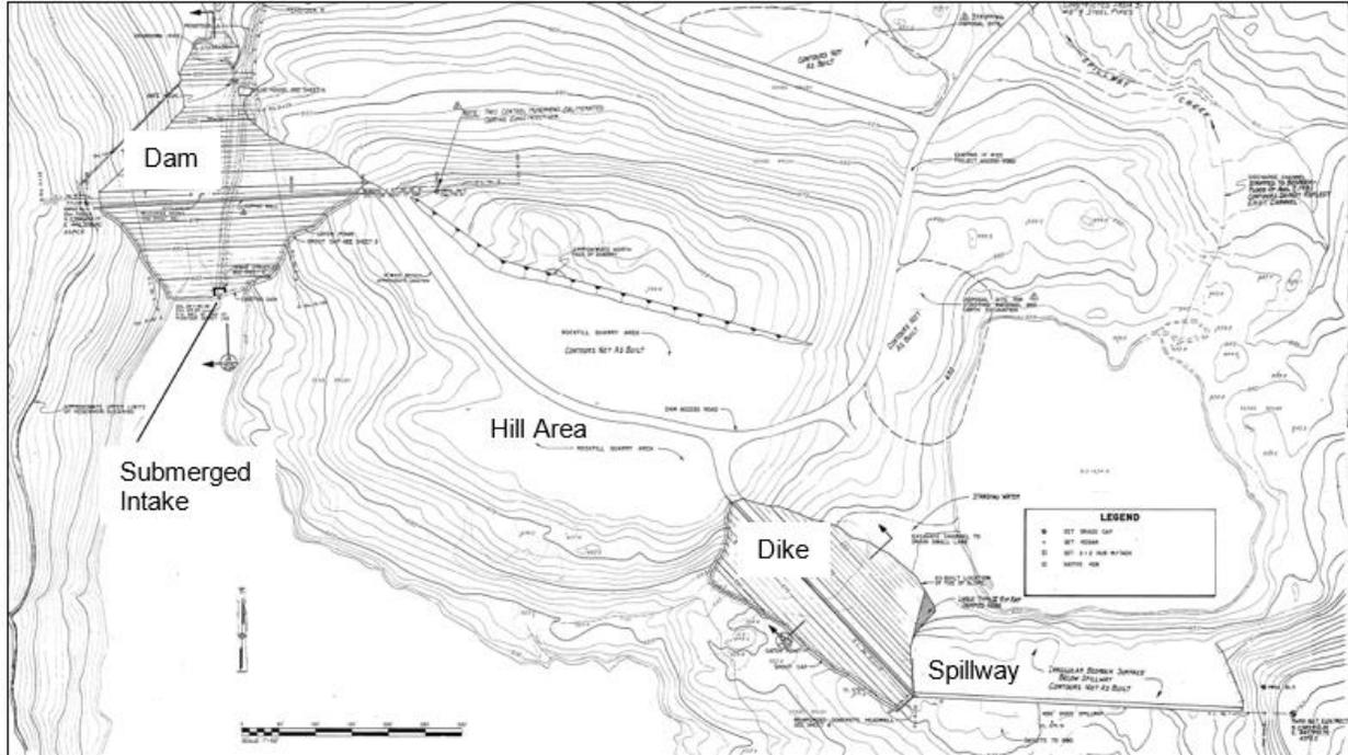
Figure 2-1. Plan view of dam, dike, and spillway
