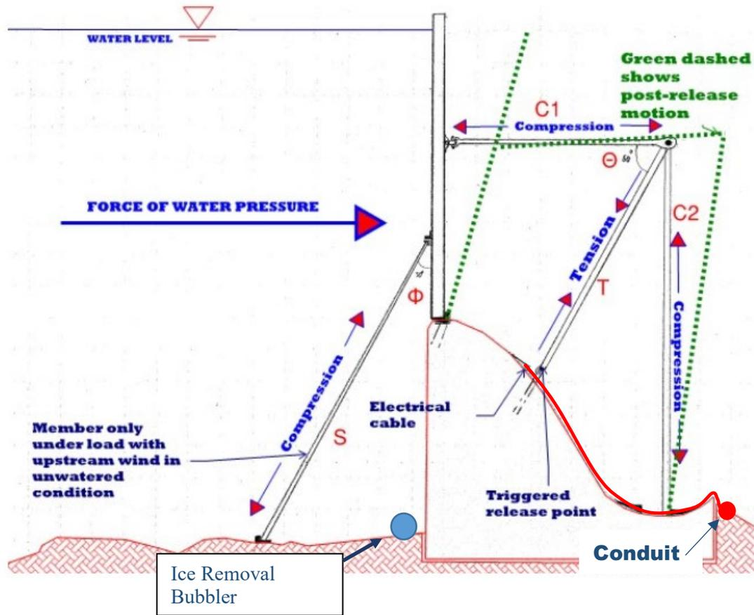
Figure D-1. Overview of components
