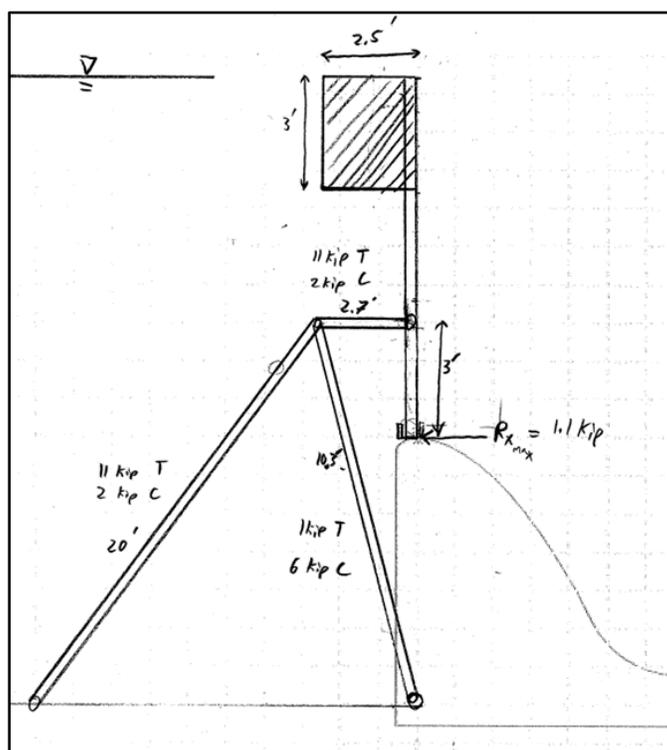
**Figure 4-5. Drawing of a vertical panel supported with a structural truss and buoyant float**
