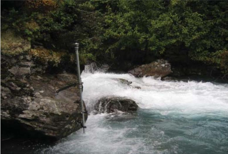
**View of one stream gauge measuring hydrology of Allison Creek.**
