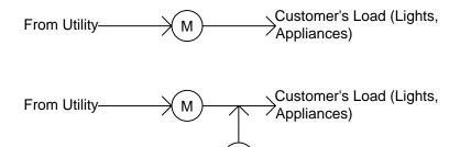
The power flowing through the meter is the Net result of the customer's load minus the customer's generation.
