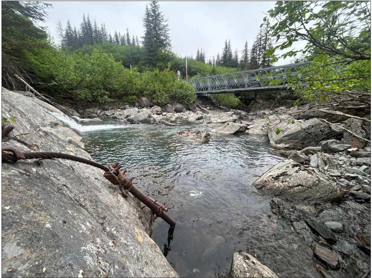
Photo 3 Thermistors attached to historic U.S. Geological Survey monitoring cable in Solomon Gulch Creek upstream of Bailey Bridge
