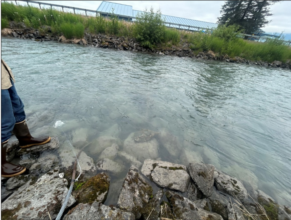
Photo 1 Two thermistors installed in the Project tailrace attached to historic U.S. Geological Survey monitoring cable
