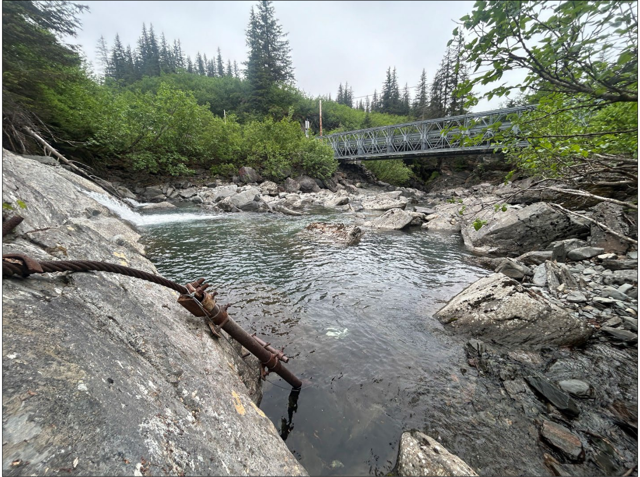
Photo 4-3 Thermistors attached to historic U.S. Geological Survey monitoring cable in Solomon Gulch Creek upstream of Bailey Bridge.
