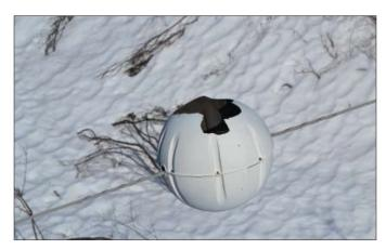
Top left, marker ball with bullet holes and frayed wire from being hit by bullets Top right, a brightly colored marker ball stands out against the surrounding terrain to demonstrate the location of the line Middle, marker balls crossing a span of line over a gorge between structures Bottom, a damaged marker ball
