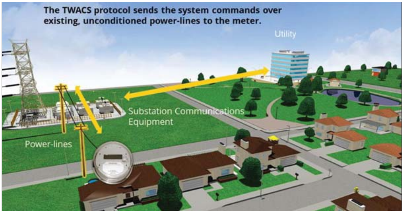
Above, the photo above depicts the flow of information using automated meters Opposite, a picture of an automated meter, similar to what will be installed on CVEA's system Photos courtesy Aclara
