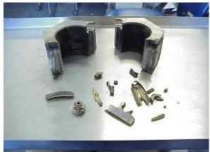
Shuttle Frangible Nut Post-Function Test
