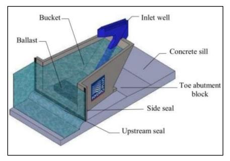
Figure 4-3. Hydraulic fuse gate manufactured by Hydroplus Corp.
