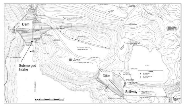
Figure 2-1. Plan view of dam, dike, and spillway
