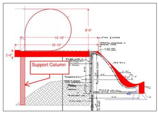
Figure 4-2. Elevation view of 8-ft rubber dam.
