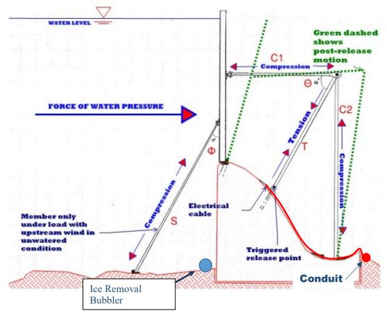
Figure D-1. Overview of components
