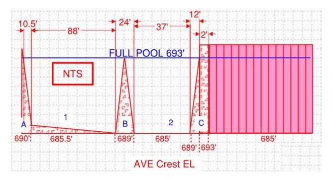
Figure C-1. Section view of compound spillway
