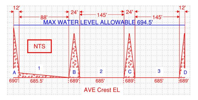
Figure B-1. Section view of deflated rubber dam at maximum allowable water level
