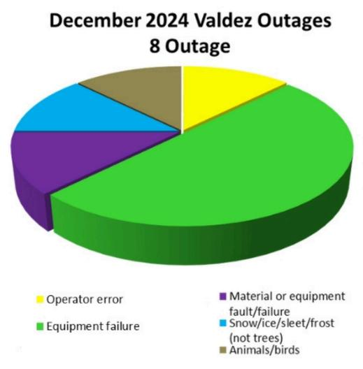
During this period, the Valdez Cogeneration unit tripped offline twice due to instrumentation failure causing two different load shed events. Since, the issue has been resolved.
