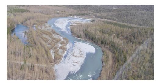
The study showed that the Tiekel drainage area was not optimal for a hydropower storage project. The terrain is lacking the ideal V notch in which to build a dam. This missing feature means a large dam is necessary to build a storage project; large dams mean high costs. Even under the best scenarios, CVEA would not be able to obtain the funds necessary to complete such a large scale project.
